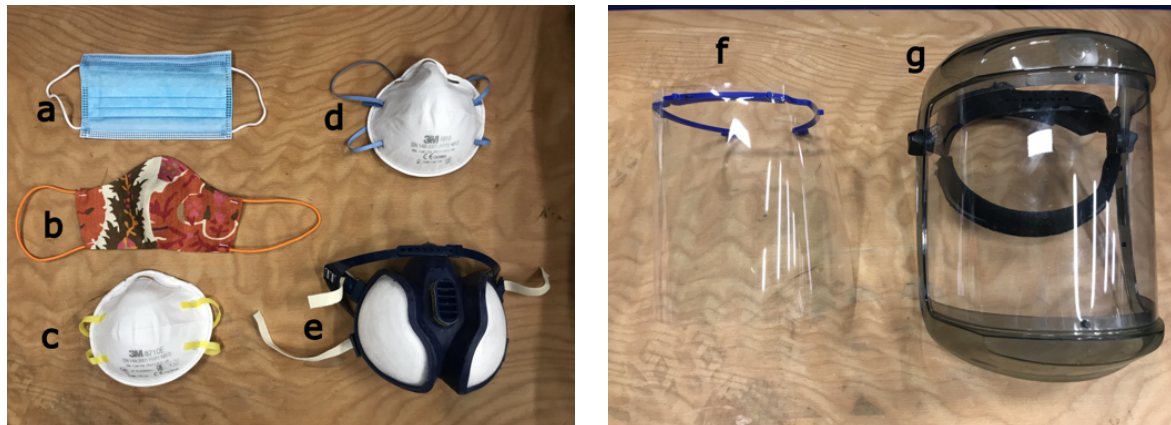
Figure 2. Different face covers tested: (a) surgical mask; (b) handmade mask; (c) FFP1; (d) FFP2; (e) respirator; (f) university-made lightweight face shield; (g) commercially heavy-duty face shield.
